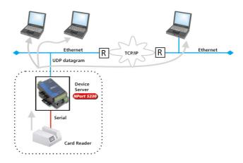
As an example, consider the situation illustrated in the above figure. In this case, the application dictates that card reader data should be sent to more than one host, all of which are connected to the Internet. The way to enforce such a requirement is to configure the device server connected to the card reader for UDP Server/Client mode, and then set up the system so that data are sent to each of the hosts.
