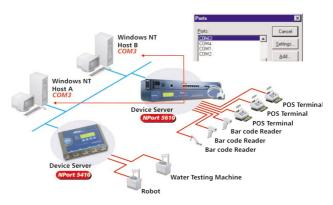
But why do we call this type of port sharing *asynchronous*? The reason is that only one host can access a port at any given time. For example, if Host B attempts to open a connection with port 1, but Host A has already opened a connection with this port, Host B's request will be denied until Host A releases the COM port. Note that this kind of application is suitable for high-security environments.
