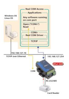
The figure shown here nicely illustrates a typical scenario of a device server configured for Single-Host application. In this case, a Card Reader is attached to a device server with IP address 192.168.127.254. The device server's Ethernet port is attached to a LAN, generally by using a straight-through Ethernet cable to connect to a hub or switch. A host computer with IP address set to 192.168.127.10 is connected to the same LAN.
