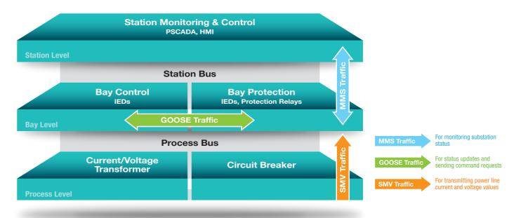
The example in the following figure illustrates how the three protocols contribute to substation communication.
