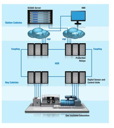
The latest development in the IEC 61850 standard was the inclusion of the PRP/HSR protocol in 2010. PRP/HSR (parallel redundancy protocol/high-availability seamless redundancy) specifies how to use two Ethernet networks to ensure seamless failover if one of the redundant networks fails.
