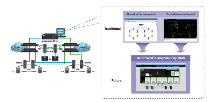
Sometimes substation networks deploy switches that do not have integrated IEC 61850 MMS, making network management more complex as these switches cannot be integrated easily into the PSCADA system. Moxa's network management software supports RESTful APIs and web widgets that enable easy integration of such devices with third-party applications (e.g., web-based SCADA).
